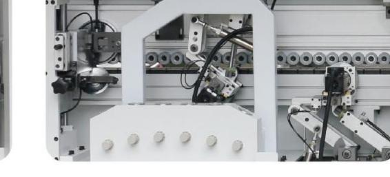
Pre-milling function The upper and lower four corners are processed to be rounded
