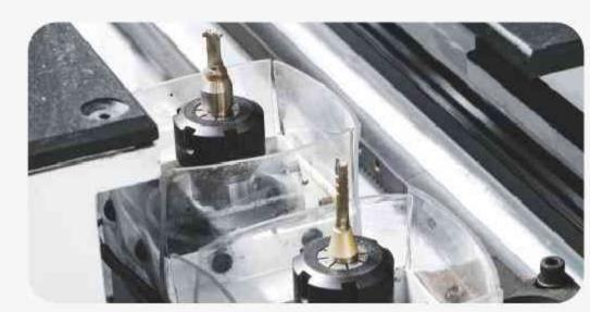
Up and down double spindle motor
