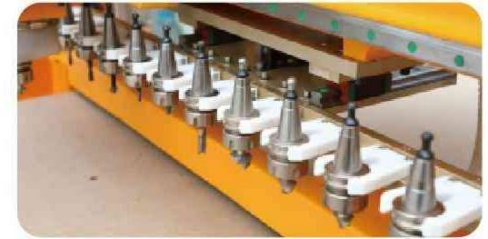
9kw spindles+12 straight tool magazine
