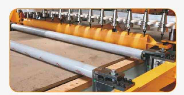
9kw spindles+12 straight tool magazine
