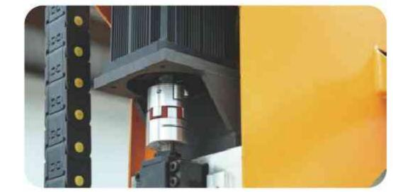
Vertical lift servo motor
