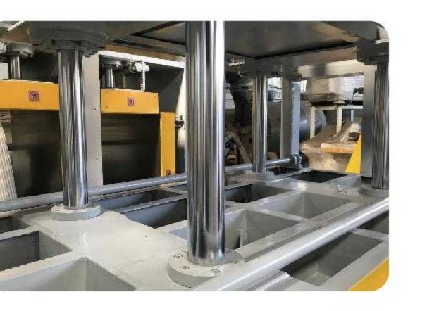
一体式油缸 Integrated oil cylinder
