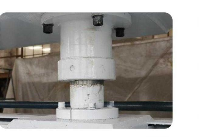
一体式油缸 Integrated oil cylinder
