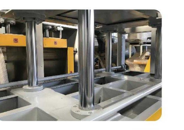
一体式油缸 Integrated oil cylinder
