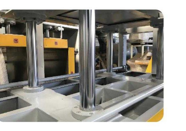
一体式油缸 Integrated oil cylinder
